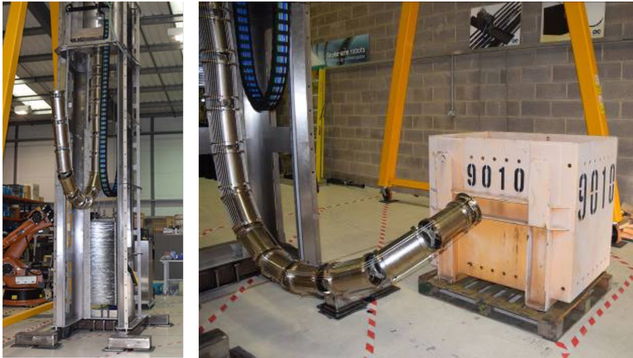
Figure 10 – Vertical deployment of LaserSnake2 system in preparation for submerged trial
