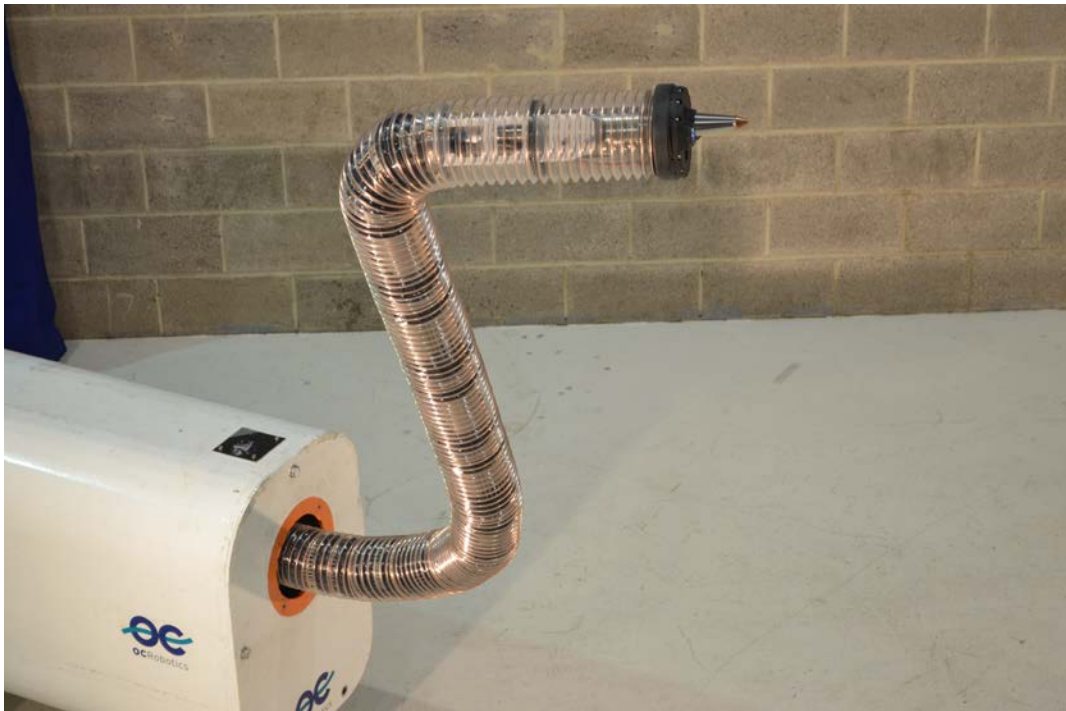
Figure 6 – Laser process head integrated with a Series II snake-arm robot
