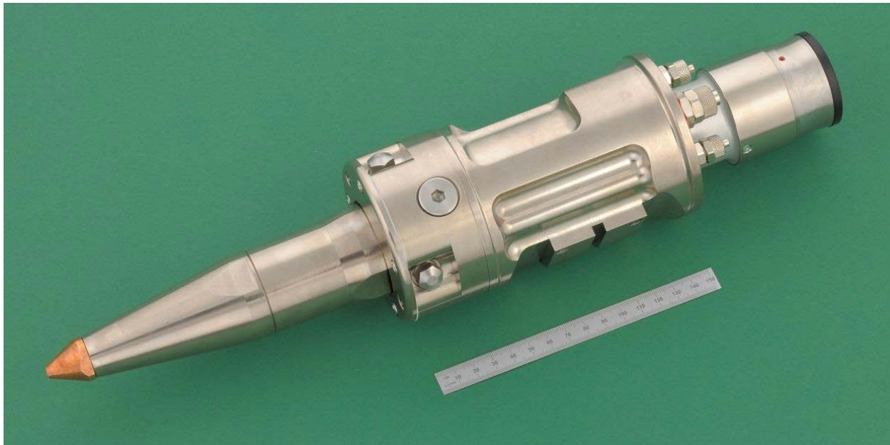
Figure 4 – Laser process head developed for the LaserSnake2 project
