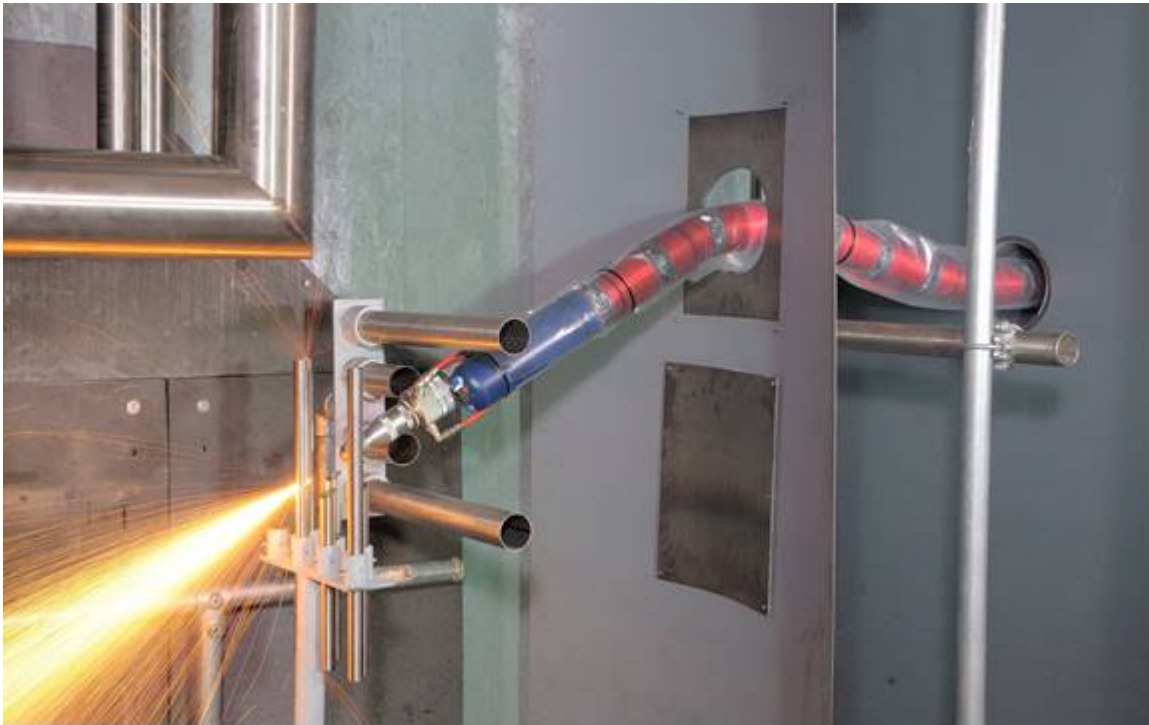
Figure 2 – Feasibility study mock-up trials of a standard snake-arm robot with a 5kw high-powered laser.
