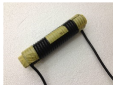
Fig. 8. receiver coil ④ (KIV3.5 sq )
