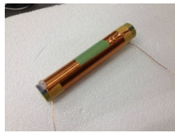
Fig. 5. Receiver coil ① (Polyester wire 0.56mm)
