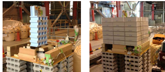
Fig. 18. Power transfer experiment (left: air as medium between coils, right: bentonite as medium between coils)
