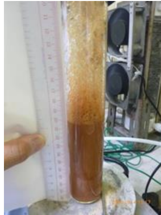
Fig. 10. Foam generated from HLLW during supplying O_3
