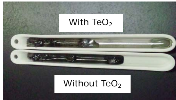
Fig. 12. The fluidity of the glass with/without \text{TeO}_2
