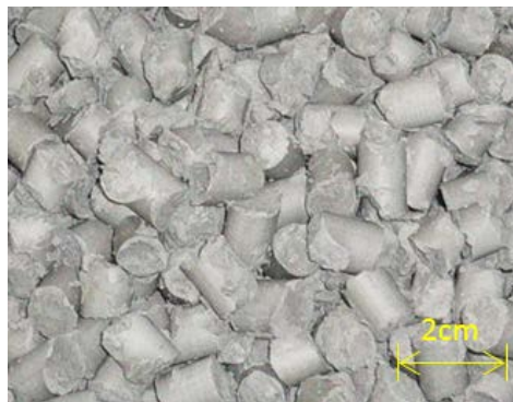
Fig. 3. Cylindrical pellets after extrusion using an 8-mm die
