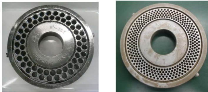
Fig. 2. Steel disks called die on which many holes are arranged. The left image is an 8-mm die with 8-mm-diameter holes and the right image is a 4-mm die with 4-mm-diameter holes.
