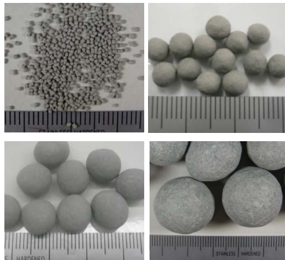
Fig. 11. High-density spherical pellets manufactured using the method described in this paper. Extrusion diameters are 1 mm, 4 mm, 8 mm, and 20 mm.
