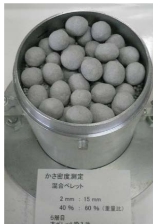
(b) Large pellets poured on the completed fourth layer
