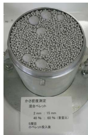
(c) Fifth layer completed after pouring small pellets
