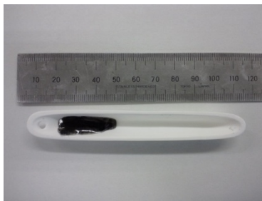
Fig. 6(a) Sample No.1 before the exam (Nitric acid nitrosyl Ru, \text{RuO}_2 0.67wt%)
