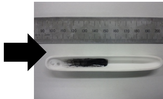
Fig. 7(b) Sample No.5 after the exam (Nitric acid nitrosyl Ru, RuO 2 0.67wt%, 40h)
