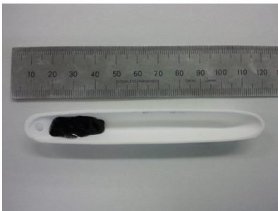
Fig. 6(e) Sample No.3 before the exam (Nitric acid nitrosyl Ru, \text{RuO}_2 10wt%)
