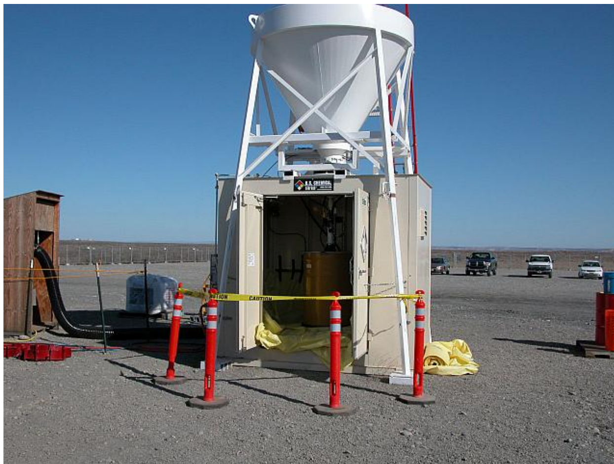
Fig. 5. Drum Opener Used at the 618-7 Burial Ground to Characterize During Remediation, April 2007.
