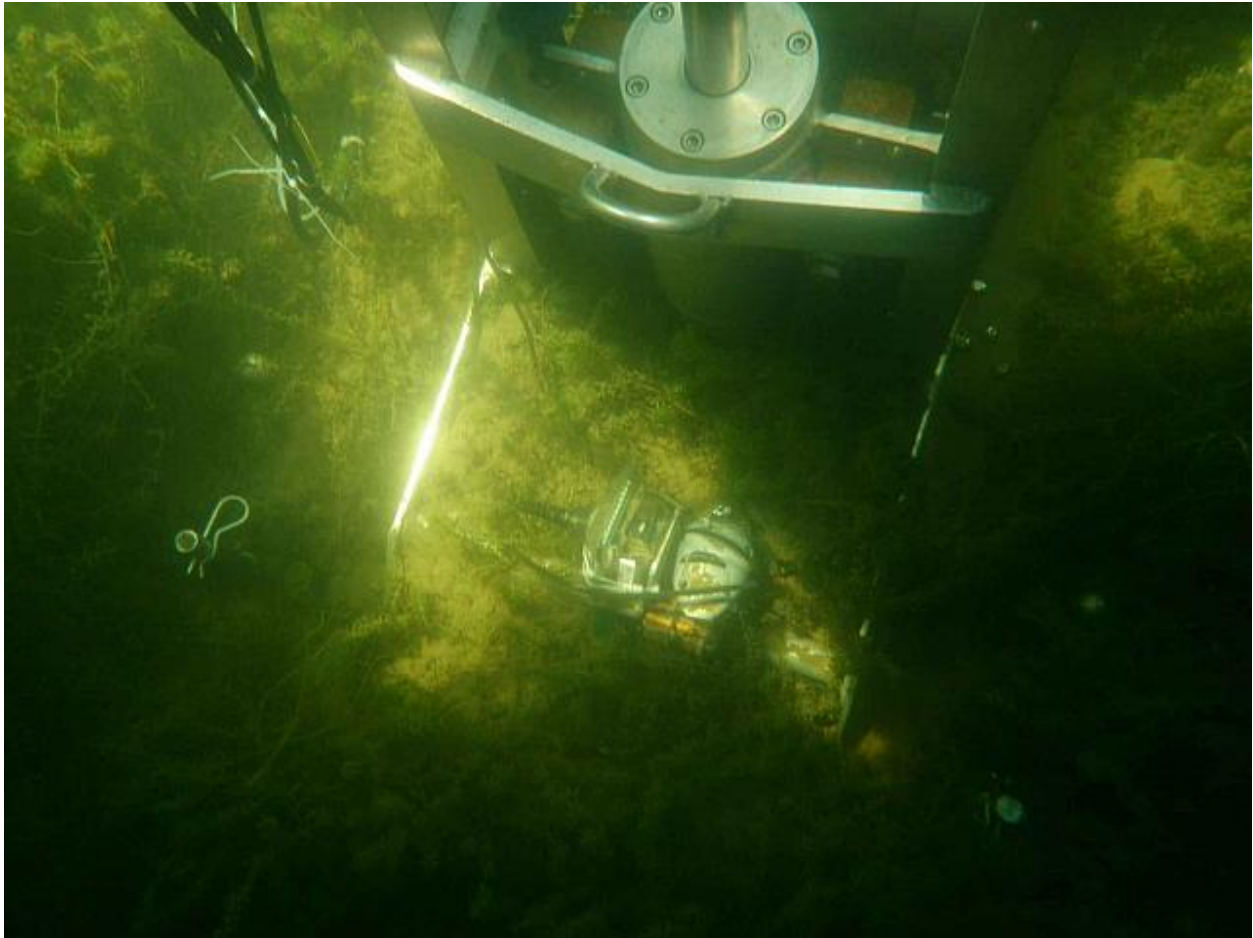
Fig. 7. A Frame Holds the Trident Probe on the Riverbed to Measure Water Temperature and Conductivity, September 2009.
