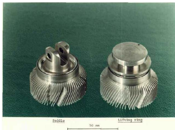
Fig. 3. Type B Tokai Mura End Crops with End Fittings in Place (Saddle, left and Lifting Ring, right)
