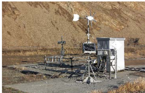
Fig. 4. Automatic Data Acquisition System at HCD-3
