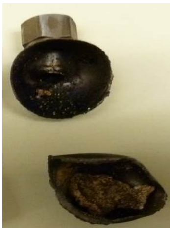
Fig. 5. ARC bomb after 7.5-g 16-h dried 3.5 M HNO 3 /sWheat experiment.
