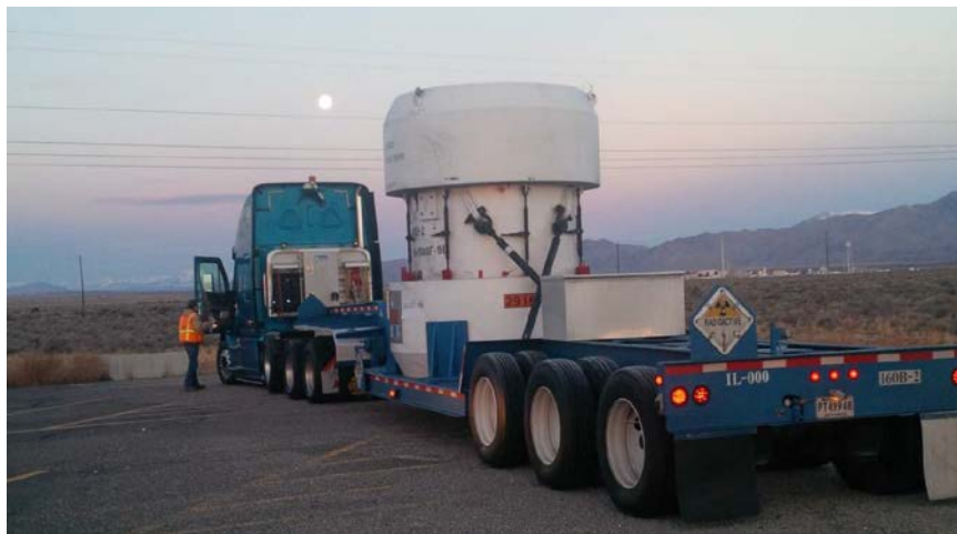
Fig. 3. A Shipment of CH TRU Waste from LANL Arrives at AMWTP for Processing
