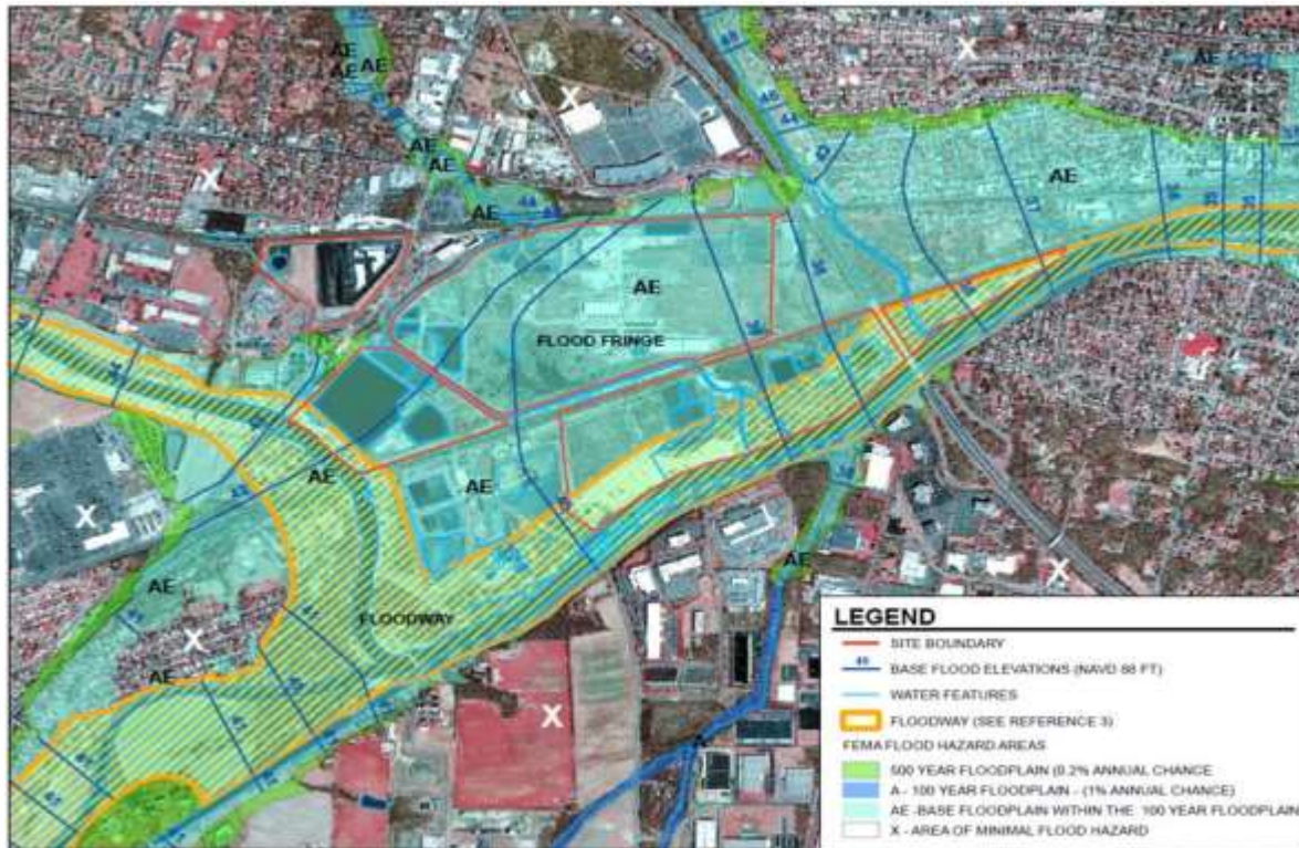
FIGURE 5. FLOOD HAZARD MAP FOR AMERICAN CYANAMID SITE WITH 100- AND 500-YEAR FLOOD PLAINS [6].
