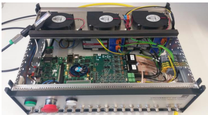
Figure 1: Ultrasonic Array Research Platform (UARP) with cover removed.
