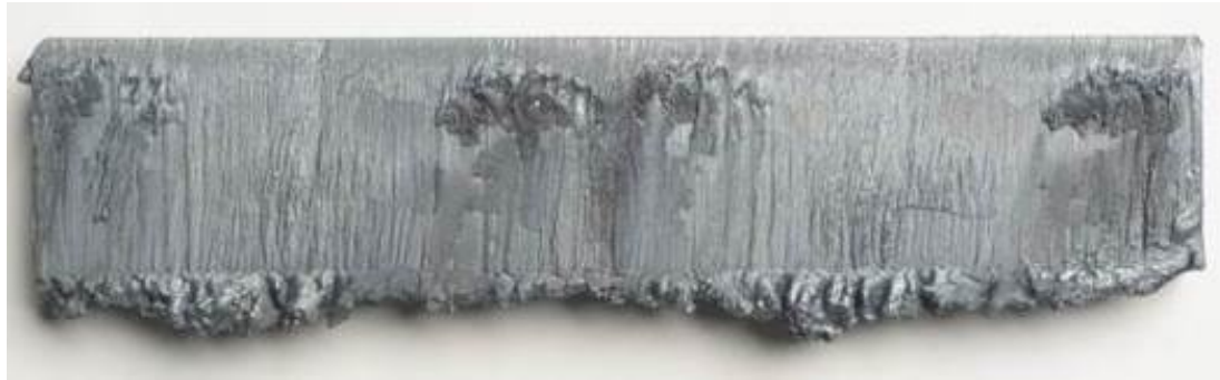
Figure 8. Cut face from a 200mm long sample of C-Mn steel cut using the 250mm lens and the DOE.
