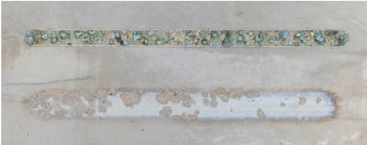
Figure 11. Effect of residual laser beam on a concrete surface. 500mm lens (top), DOE plus 250mm lens (bottom), for the same laser power, beam focus to concrete distance and travel speed.
