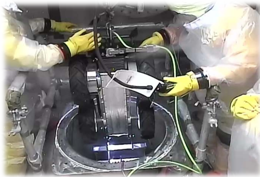
Fig. 16. Vertical Insertion of the RC through the Manway
