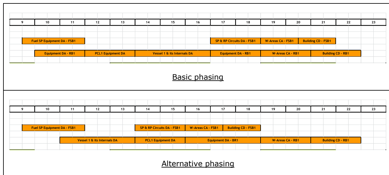
Figure 3. Phasing of dismantling actions in the RB and FSB (all NPP's units)
