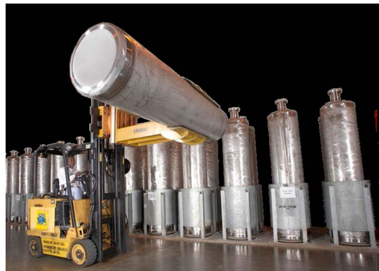
Defense Waste Processing Facility HLW Glass Canisters
