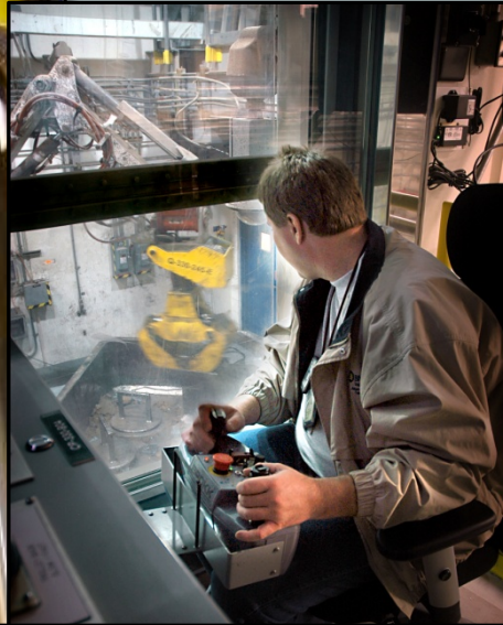
Business end of Supercompactor = > 4 million pounds of pressure
