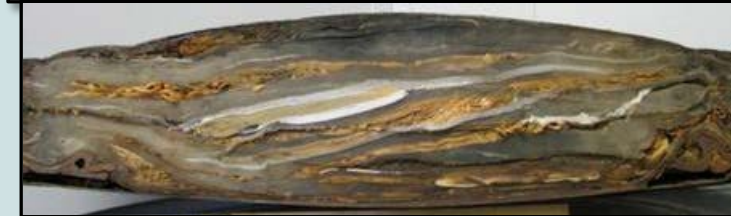
55-gallon drum post Supercompactor = a puck
