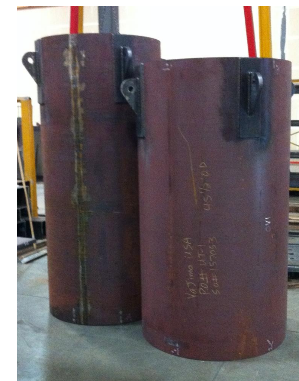
Overpacks of Cask I and Cask II
