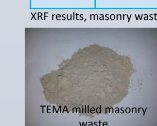
vitrified masonry waste, 68 wt% SiO 2 (masonry waste), 18 wt% B 2 O 3 , 14 wt% Na 2 O
