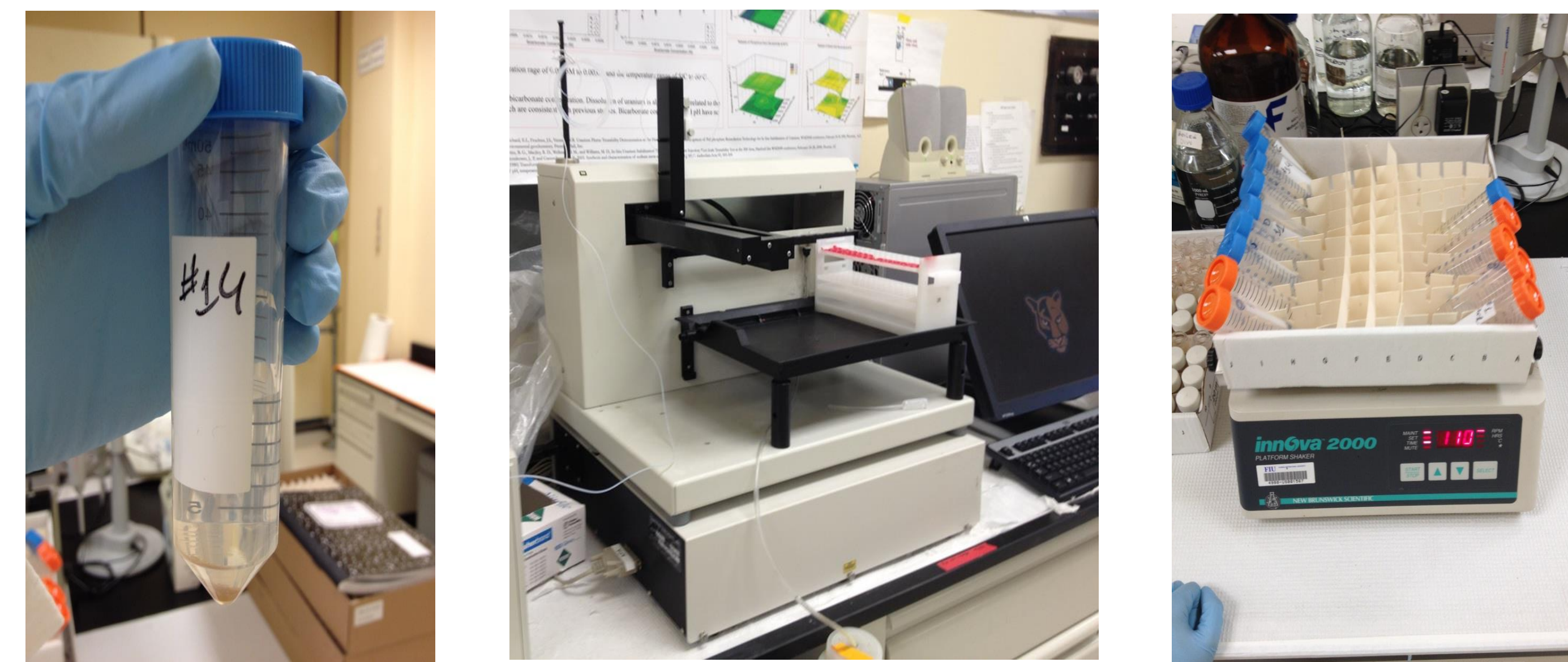
Figure 2. Experimental sample, KPA Instrument, platform shaker used throughout the experiment
