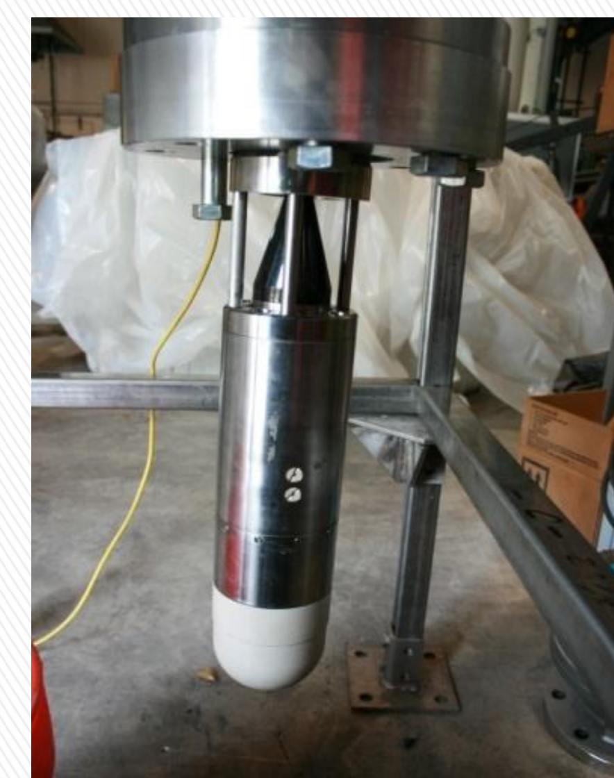
Figure 3: Solid Liquid Interface Monitor (SLIM) 3D Sonar
