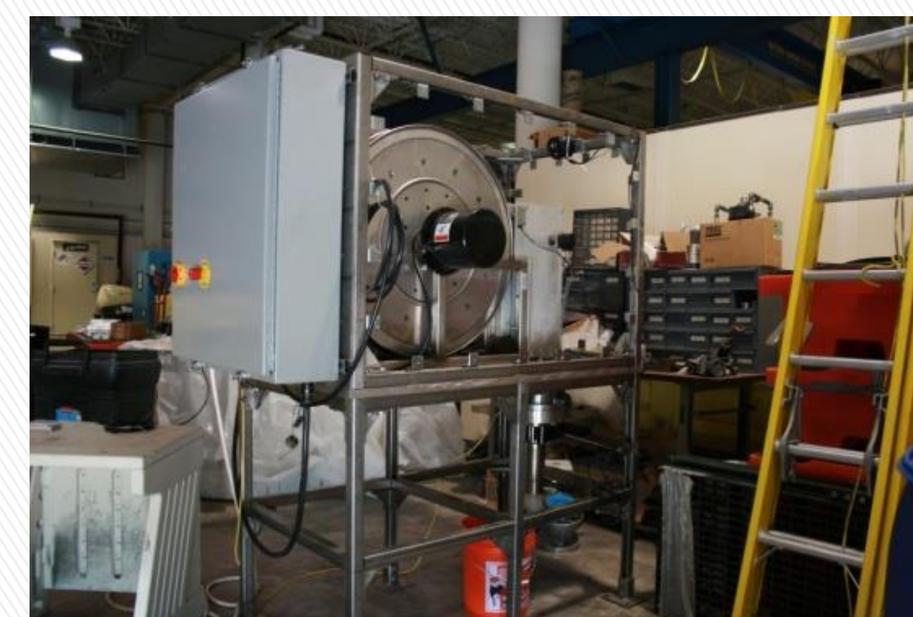
Figure 2 : SLIM's deploying mechanism for 75-ft diameter tanks
