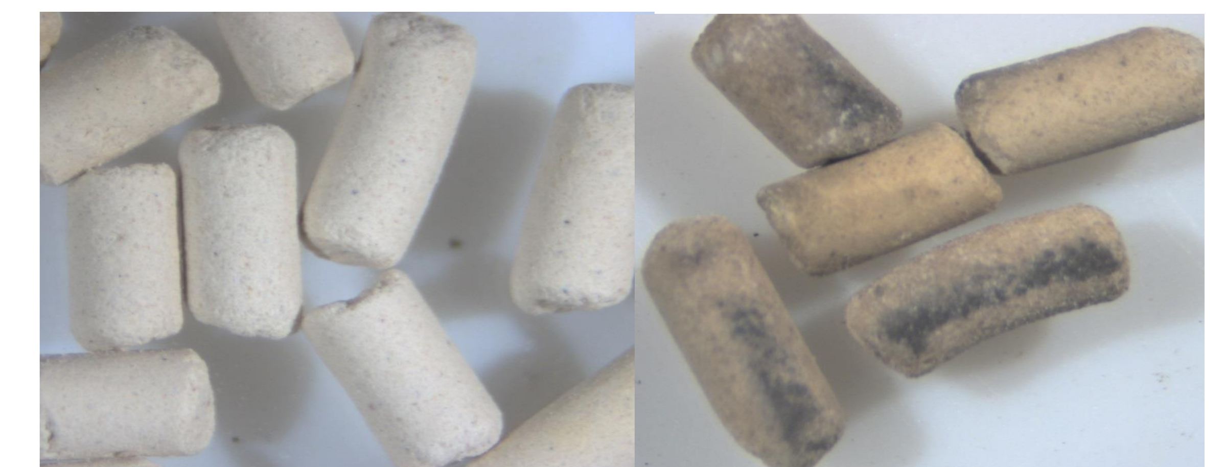
Pictures of Ag-mordenite pellets before ( left ) and after ( right ) the test with KI
