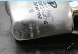
Physical results showing actual deformations. Side drop slap down (Left) and Penetration test near collar (Right)
