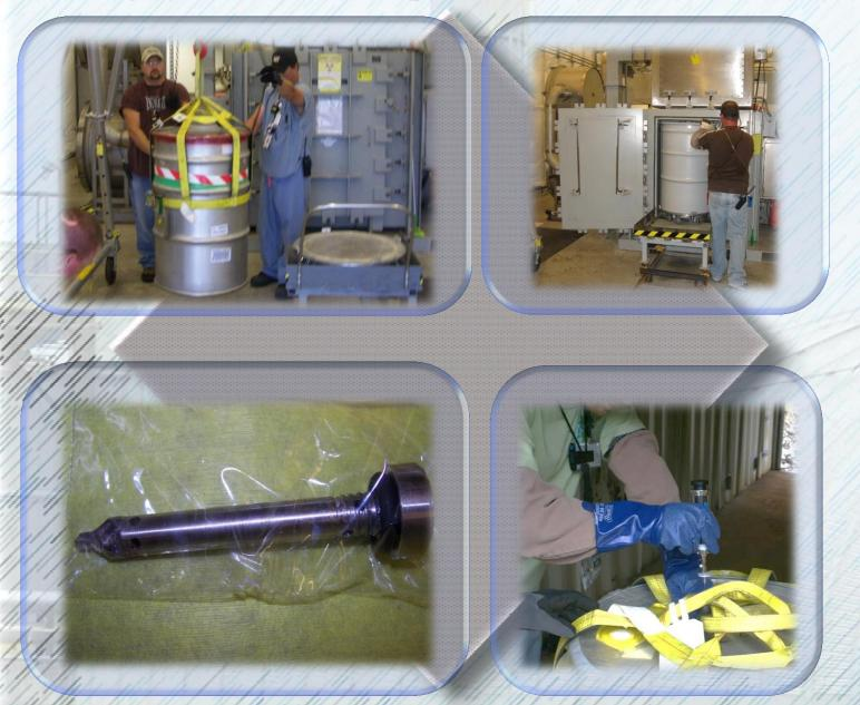
The Remote Drum Opener (RDO) system was designed, tested and placed in service to vent drums discovered in overpack boxes and to vent overpack configurations (e.g., 110 gallon overpacks and multiple drum configurations).
