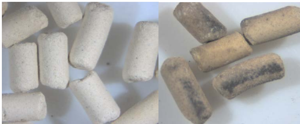
Fig. 6. Pictures of Ag-mordenite pellets before ( left ) and after ( right ) the test with potassium iodide
