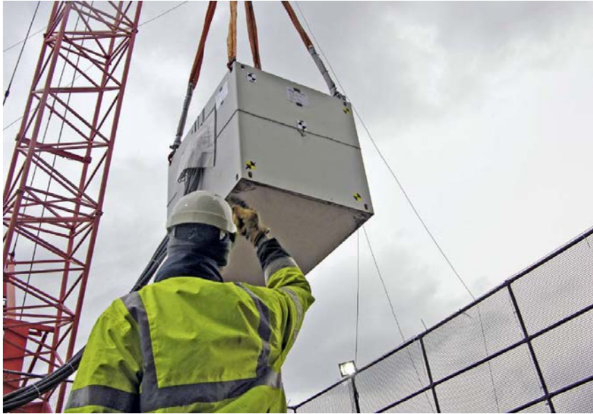
Fig. 5. Drop test of 5.2 m at Winfrith Drop Test Facility, UK, for the BlueBox®
