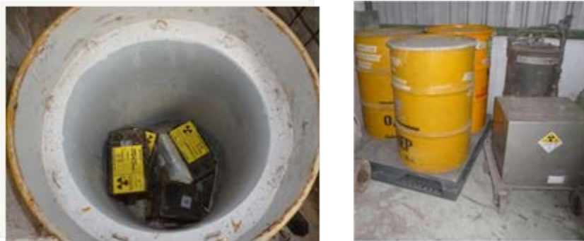
Figure.6 Re-packing of DSRS in 200 Liter Drum
