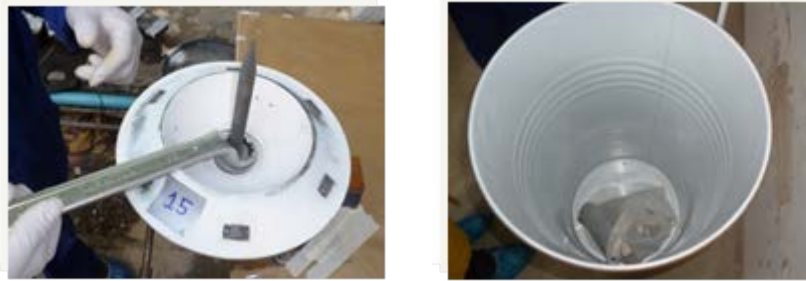
Figure.5 Volume reduction by removing DSRS from big containment and re-packing
