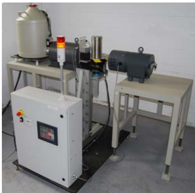
Fig. 1. Canberra's Can-TGS System for Small Containers
