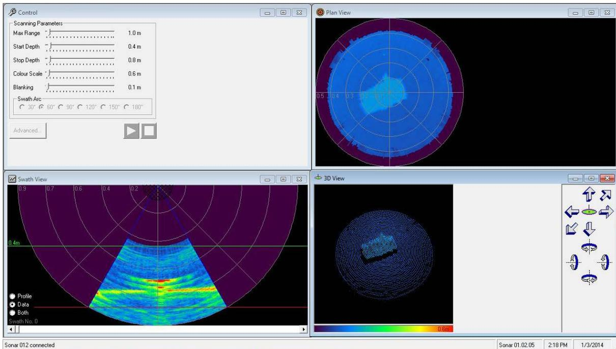
Fig. 4. High resolution image using sonar manufacturer's graphical user interface. The 4 views include: sonar settings (upper left), top view (upper right), side view (lower left) and a 3-D map of the brick in the bottom of the test tank (lower right).
