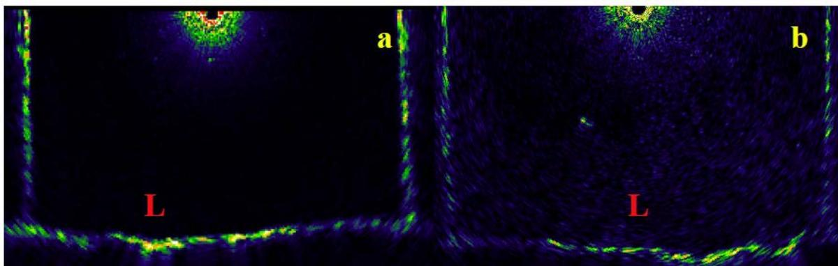
Fig. 3. 2-D Sonar Image of 30 cm of settled kaolin on the floor; a) without mixing; and b) with mixing such that 30% of the liquid volume was from entrained solids. Radius of the tank,  $L$ , is 109 cm.
