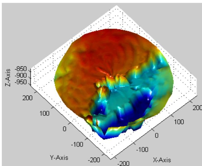
Fig. 8. 3-D Sonar Scan for: 30 Degree Swath Arc; 29 seconds; and 3% vol. Kaolin
