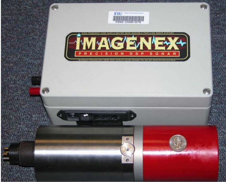
Fig. 1. Custom-built 2-D Profiling Sonar at FIU.
