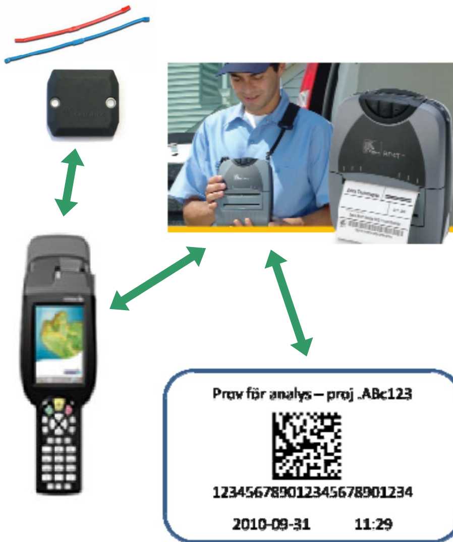
Fig. 7. Equipment for documentation of sampling position in the facility.
