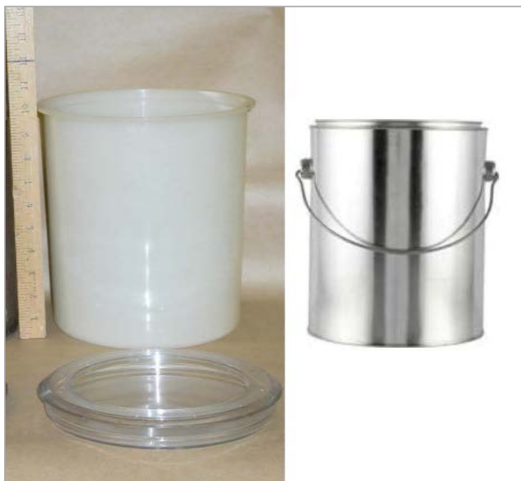
Fig. 2. Typical 7-inch plastic can and 1-gallon, metal cans used to remove waste from hot cells. Lids were not used on metal cans until 1987.
