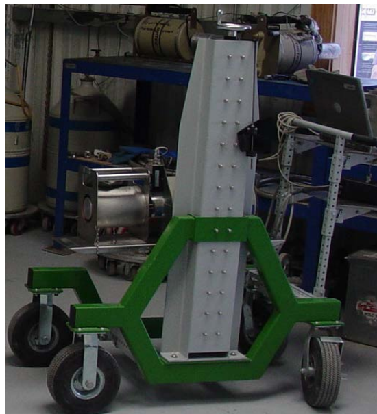
Fig.1. Portable far-field HPGe detector system.
