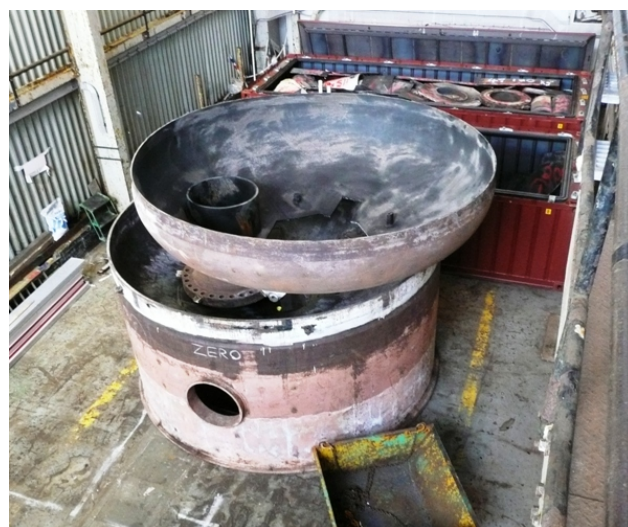
Figure 14: Cleaned DDT Top and Bottom Domes
