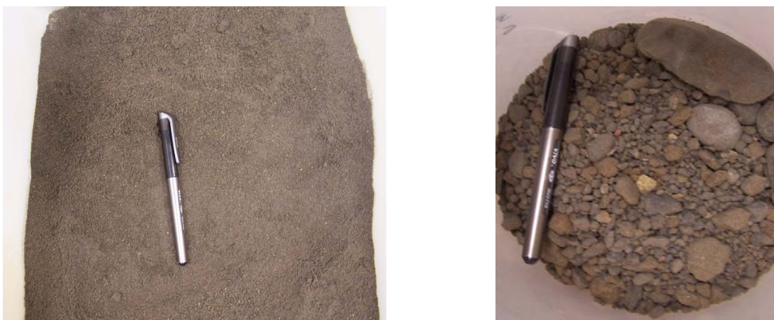
Figure 2. Hanford sediment passing No. 18 sieve (left) and retained on No. 18 sieve (right).
