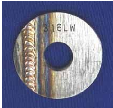
Fig 13. Welded Corrosion Coupon, courtesy of Metal Samples Company ( www.metalsamples.com )
