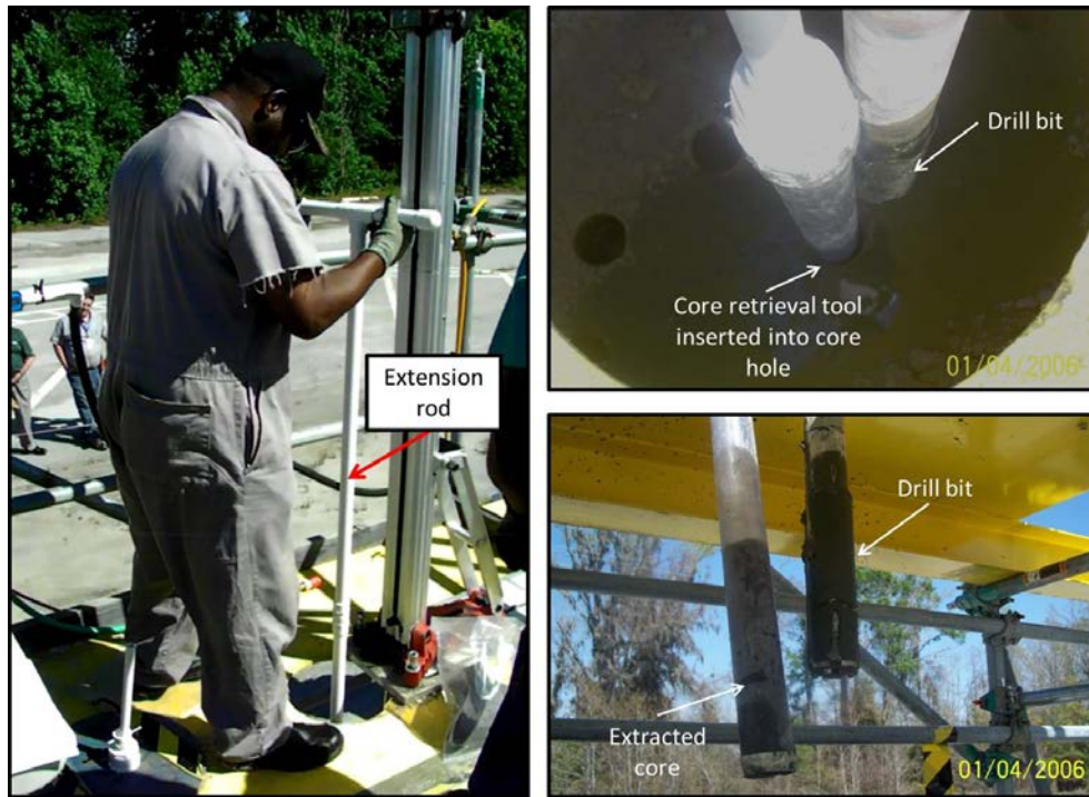
Figure 9: Core extraction utilizing the purpose-built core retrieval tool.
