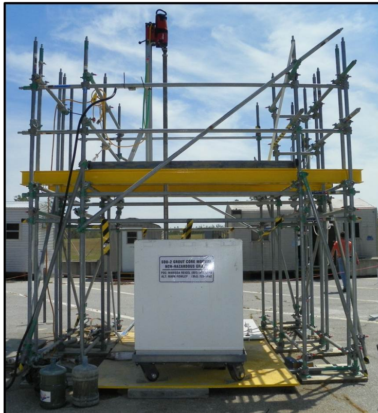
Figure 4: Dedicated test stand for SDU core-drilling mock-up.
