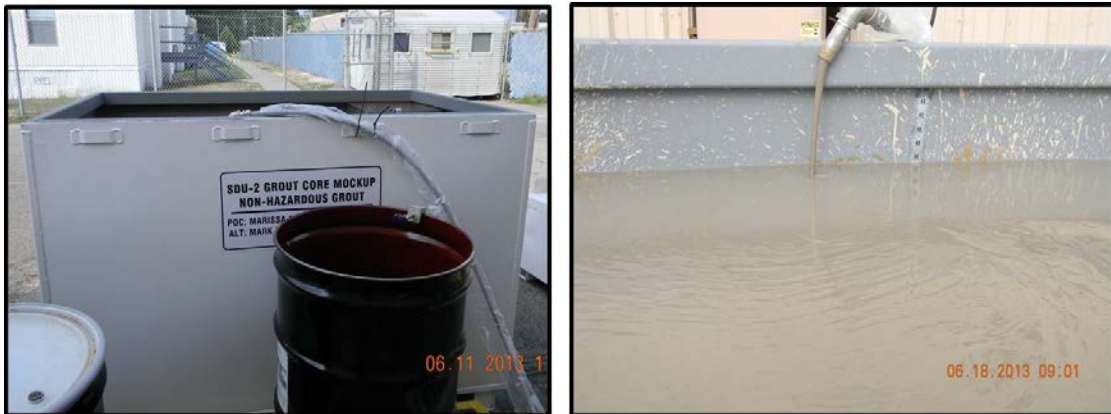
Figure 1: Photos illustrating the filling of a B-25 container with simulant saltstone.
