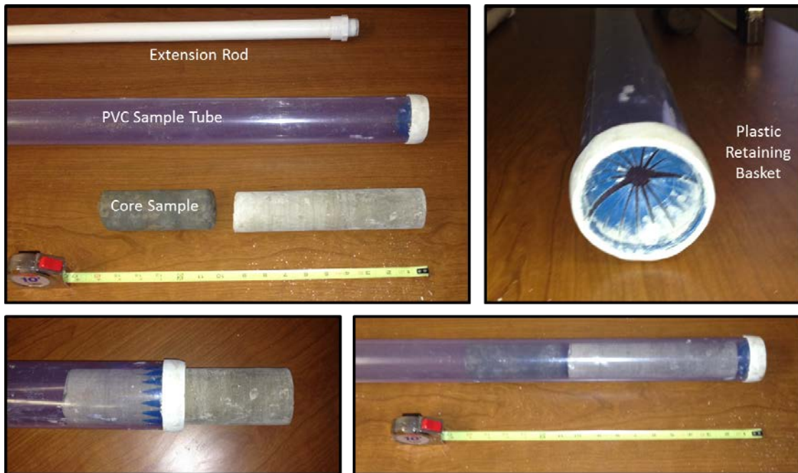
Figure 6: Photographs illustrating the core retrieval tool.
