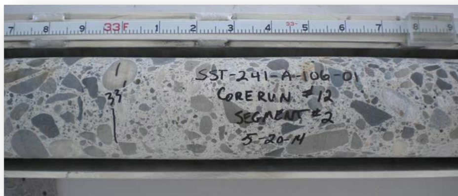
Fig. 5. Example Concrete Core Photo from Tank 241-A-106 Sidewall (33 feet)
