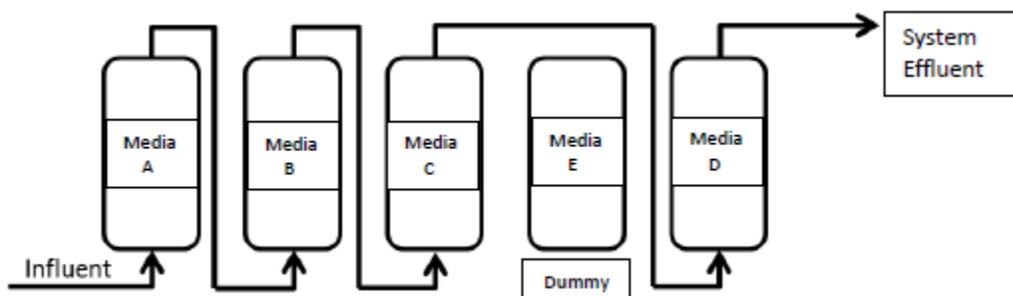
Figure 4: KMPS 8 Day Column Rotation Configuration for TS-G
