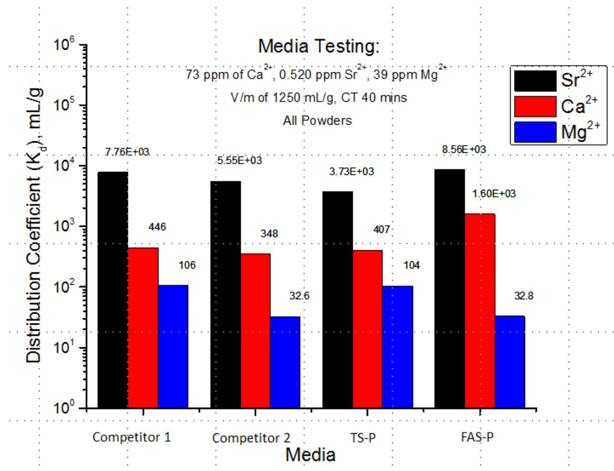
Figure 3: Shortened Contact Time Batch Test Comparison (Competition vs Kurion Media Example)
