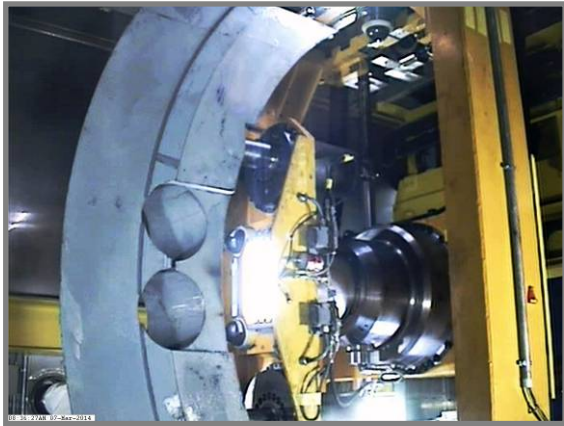
Fig. 5 Lifting up of a primary shielding block
