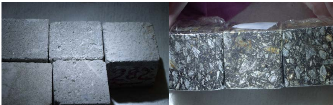
Figure 1. Typical coupons of concrete (left) and asphalt (right).
