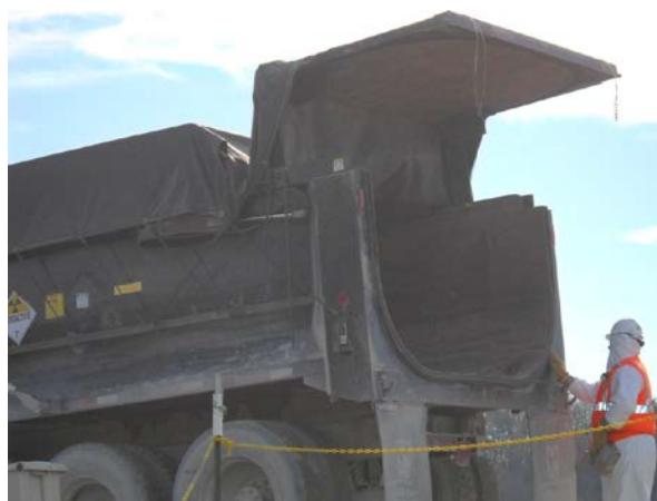
Fig. 8. Dump Truck Being Surveyed at Decontamination/Survey Station
