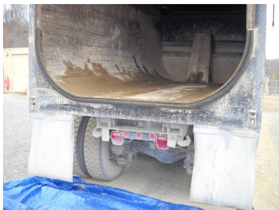
Fig. 7. Dump Truck Showing Gasket Used for Contamination Control
