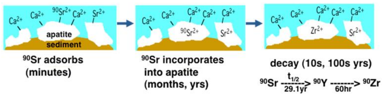
Fig. 4. Strontium Substitution for Calcium in Apatite Matrix.
