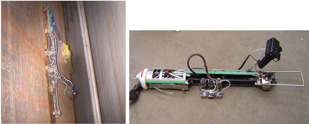
Figure 3. (a) In-Use P-scan Wall Crawler (b) Top View of the P-san Wall Crawler.
