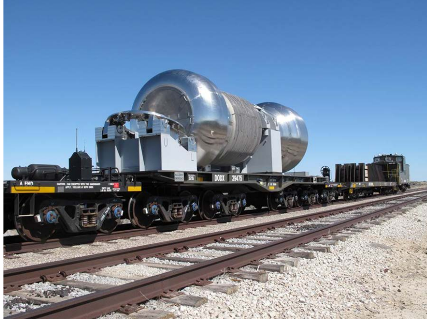
Fig. 3. US Navy AAR S-2043 Compliant Railcar with Cask (Not for transport of commercial SNF).
