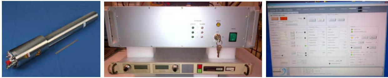
Figure 5. Photographs of the SODERN Genie 16 NG system showing the NEM (LHS), Control Chassis and VHV power supply (Centre) and the System's Software Interface (RHS)
