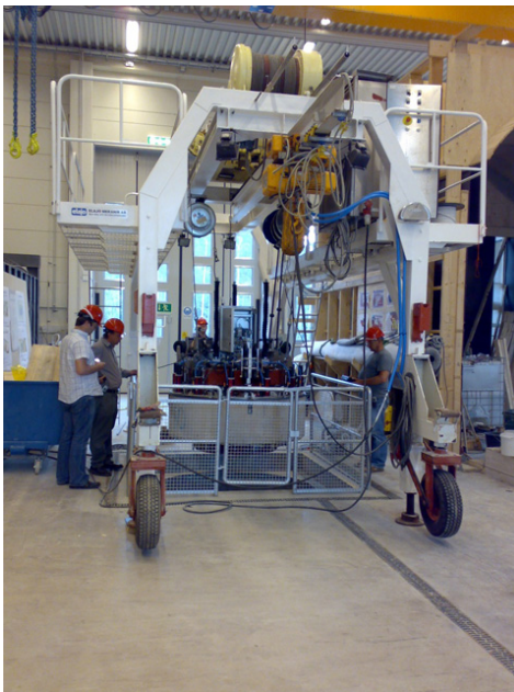
Fig. 4. Testing of installation of buffer blocks in the Bentonite Laboratory.
