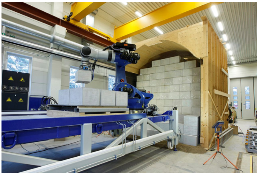
Fig. 5. Testing of installation of backfill blocks in the Bentonite Laboratory.
