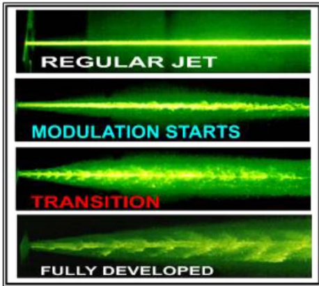
Figure 1 – High speed photographs of a traditional water jet and the establishment of a FPWJ.
