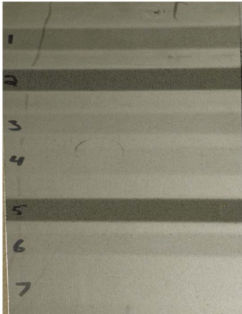
Figure 6 – Shows the banding effect from changing parameters, against a series of trial runs. Darker bands show greater degrees of erosion that correspond to more overlap (equivalent to jet dwell time).
