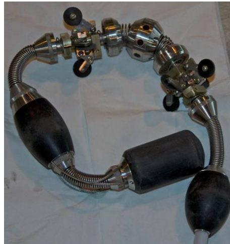
Fig. 3. Coil Thickness Inspection Device
