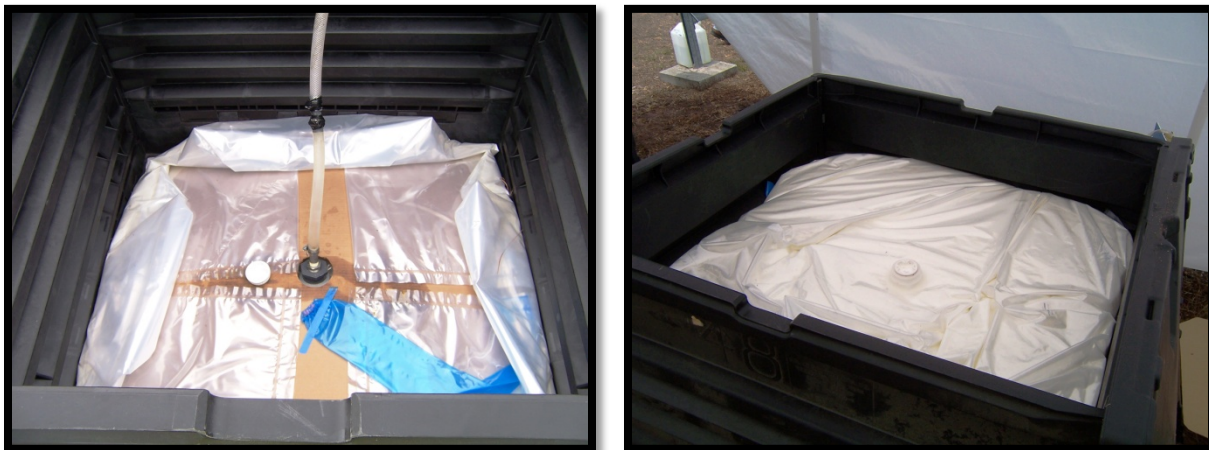
Figure 5: Photograph of a Tote Before (left) and After (right) Filling with Groundwater and Amendments
