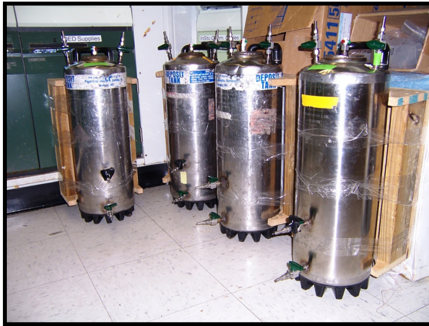
Figure 4: Photograph of Canisters Containing the MicroCED
