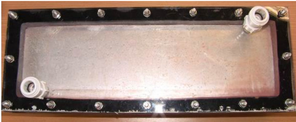
Figure 9a A small scale narrow cavity (nominally 120mm high, 400 long and 22mm thick)
