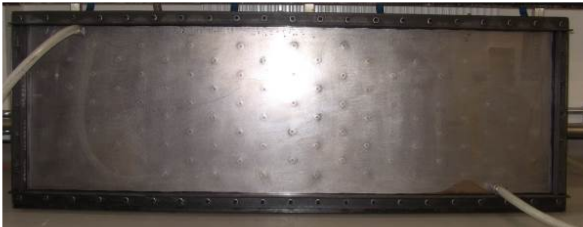
Figure 9b A narrow cavity (nominally 600mm high, 2000mm long and 22mm thick). Both cavities have one adiabatic wall and the other wall kept at 40°C. By changing the direction of flow of the ice pig the capability of the ice pig to remove debris and loose rust from the floor area was investigated.
