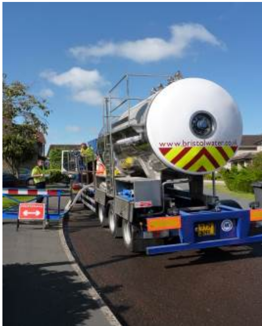
Figure 10 The ice-pig delivery lorry ready to undertake a live trial
