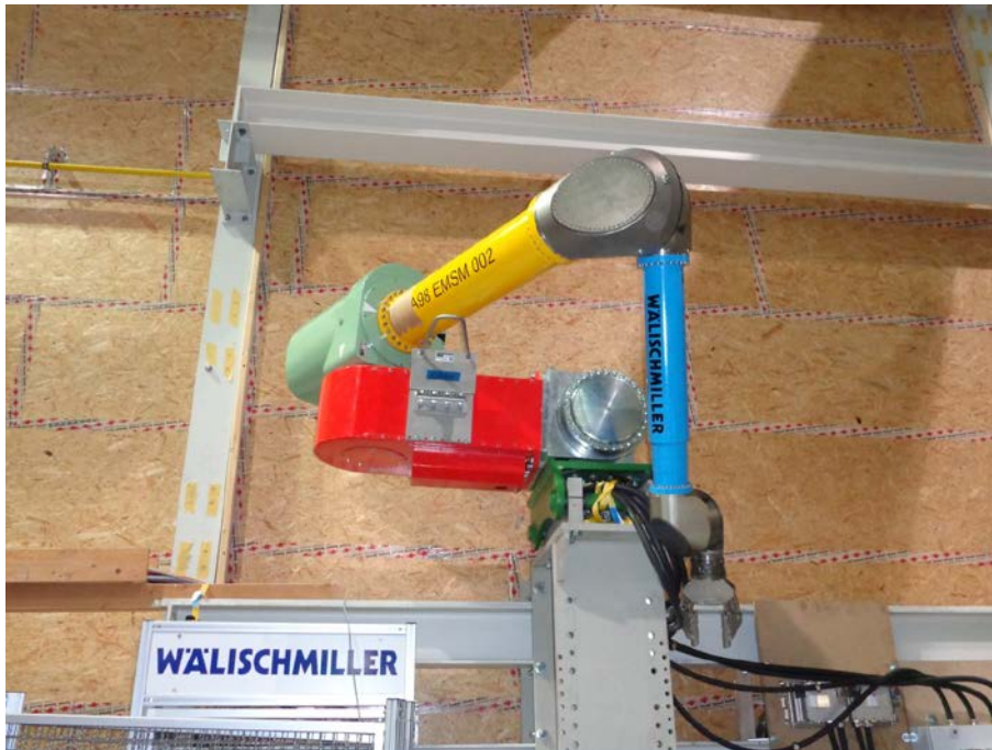
Fig. 16. Mock-Up for testing overhead working positions
