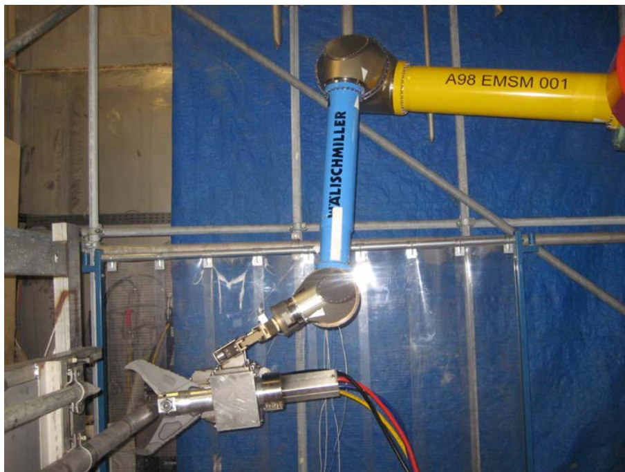
Fig. 11. Measuring the back lash of the tools
